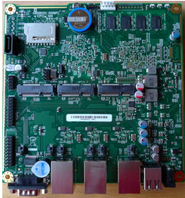
Figure 2: The APU system board we use as base node. We design the MONROE hardware around it by adding several accessories.
