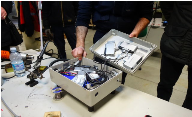
(a) Assembled mobile MONROE node, showing components fixed inside white box enclosure.
